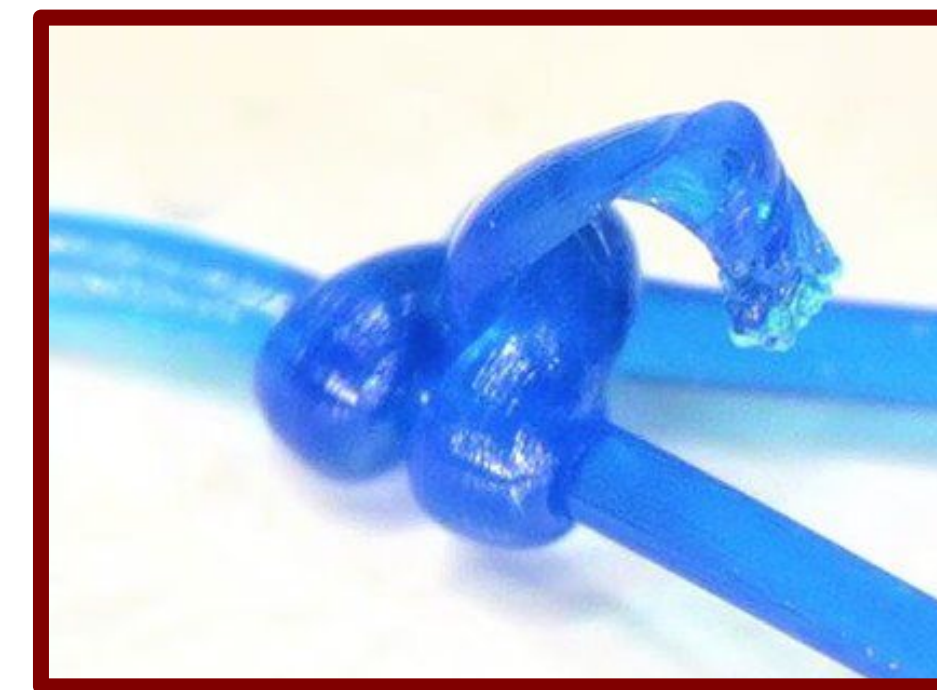
Figure 2: Suture material failure from over tightening [2].
