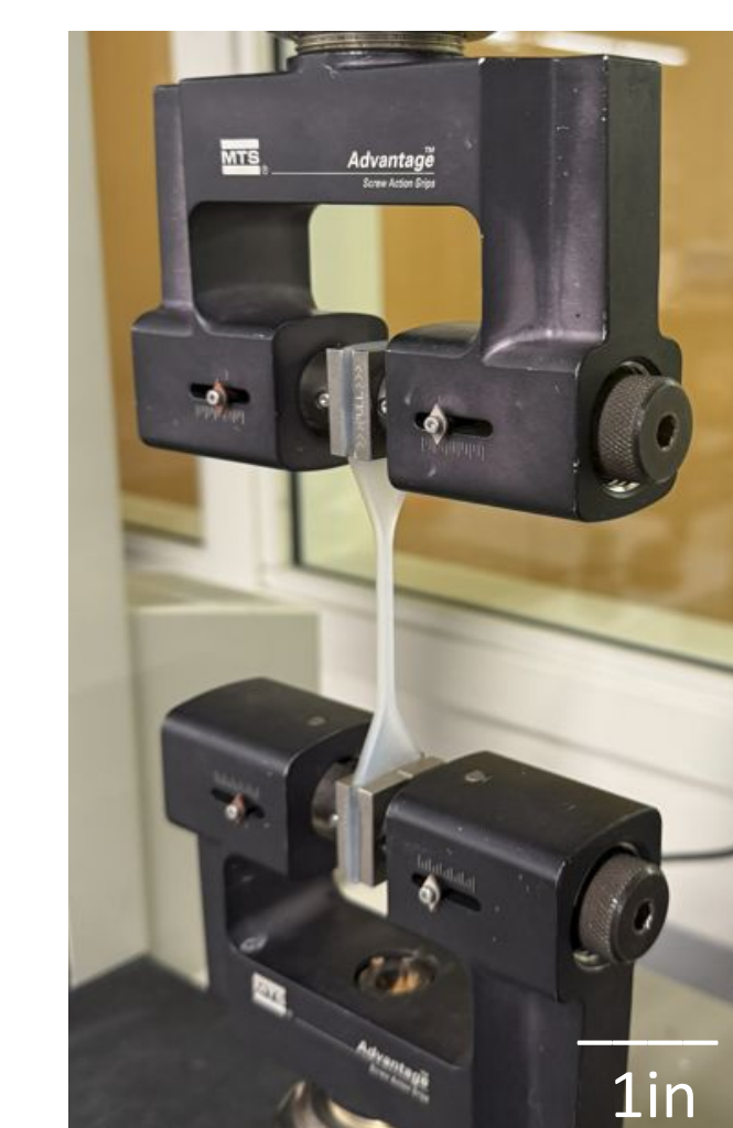
Figure 7: MTS Testing of Ecoflex 00-20
