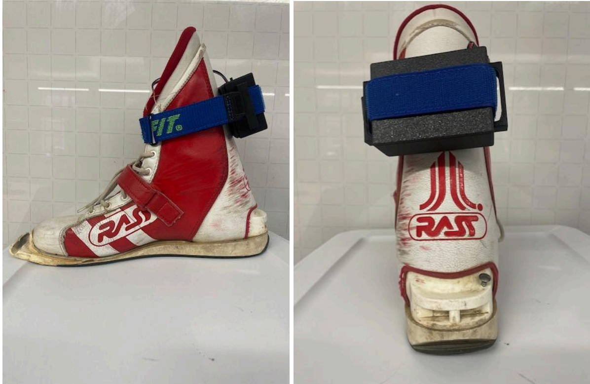
Figure 14: Final circuit design with the housing unit attached to a ski jumping boot via a velcro strap.
