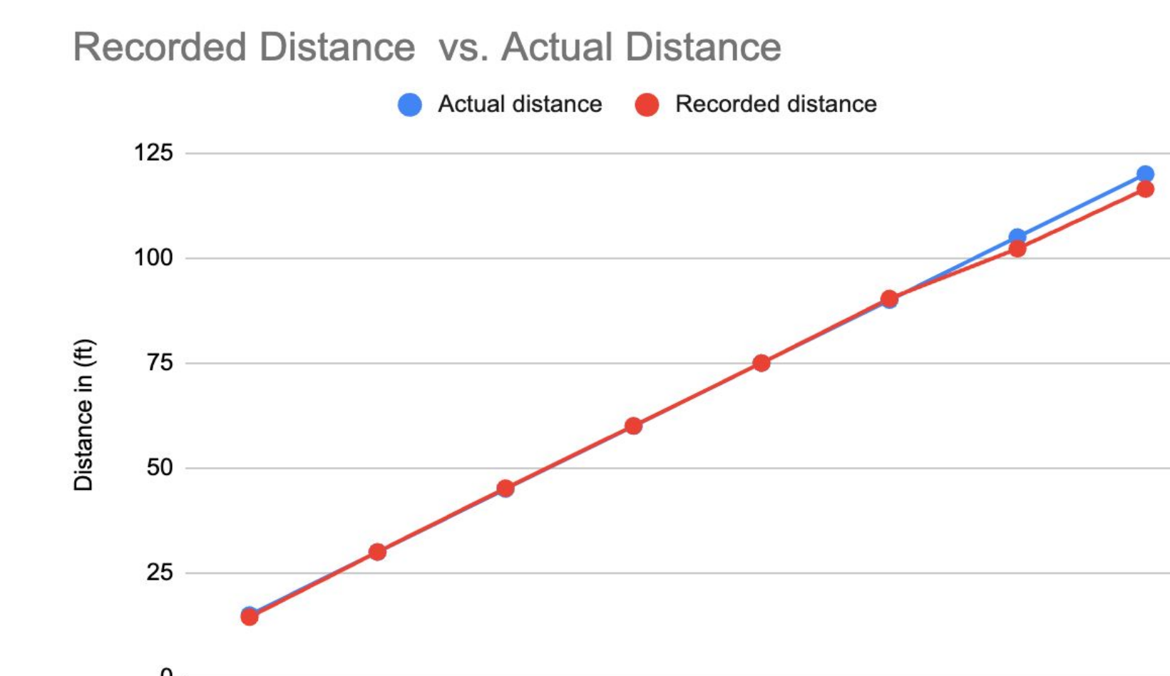
Figure 7: Lidar Validation Testing
