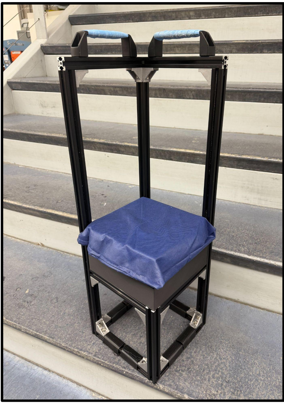
Fig 2. Final Knee Crutch Prototype, shown with the 5cm adjustability block
