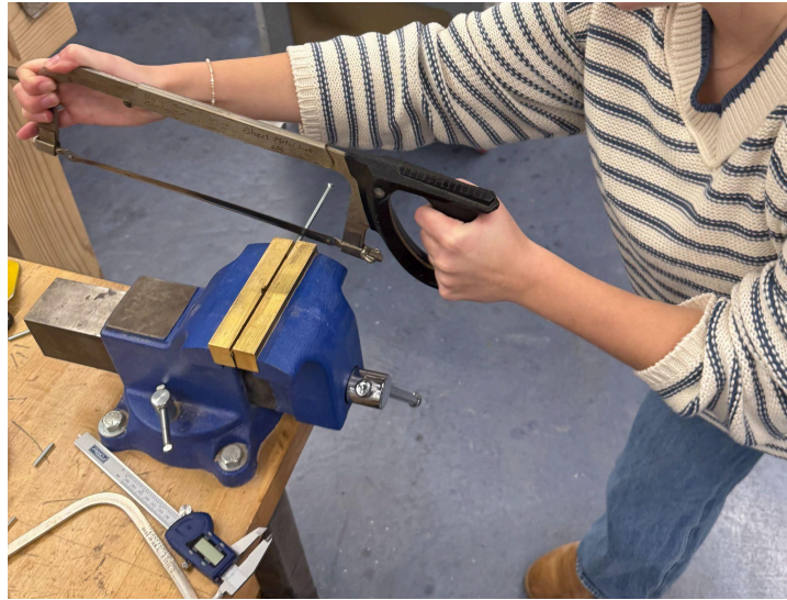
Figure 5. Hacksawing a screw down to size using a bench vice
