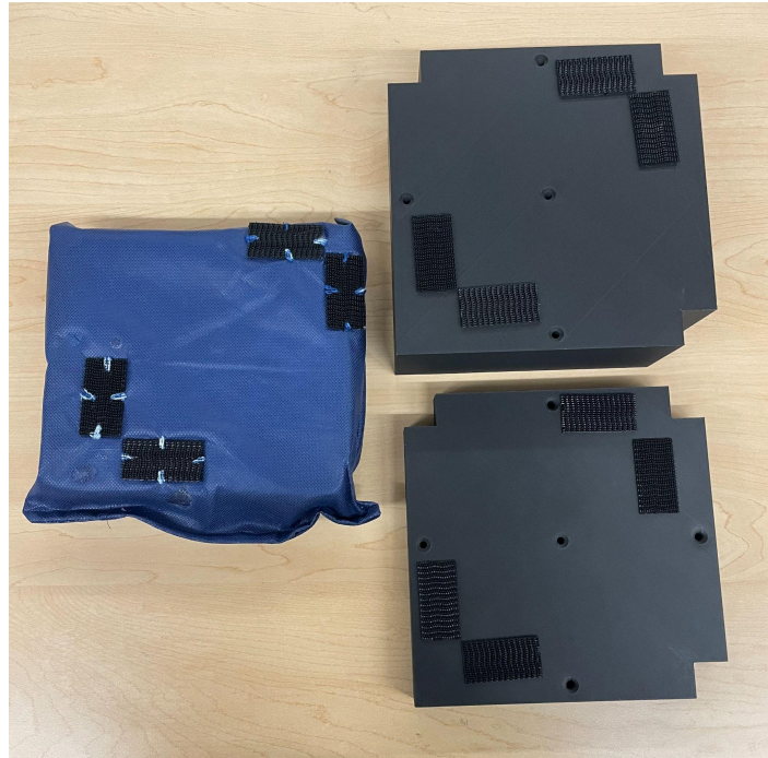
Figure 8. Two adjustability blocks shown side by side with the velcro-compatible cushion (Top Right: 2.75" block , Bottom Right: 1" block, Left: bottom face of cushion)
