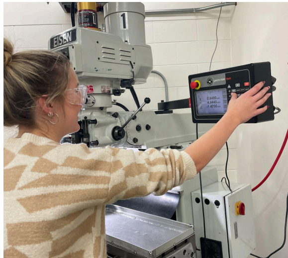
Figure 3. Zeroing out the mill to begin sizing the aluminium rods
