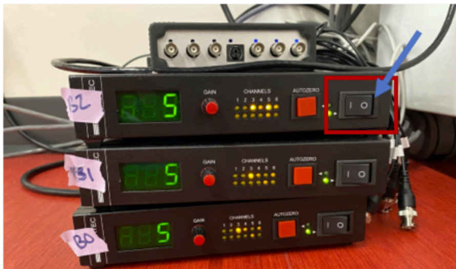
Figure 7: Amplifier boxes for in-ground force plates with indication of the power switch [o]
