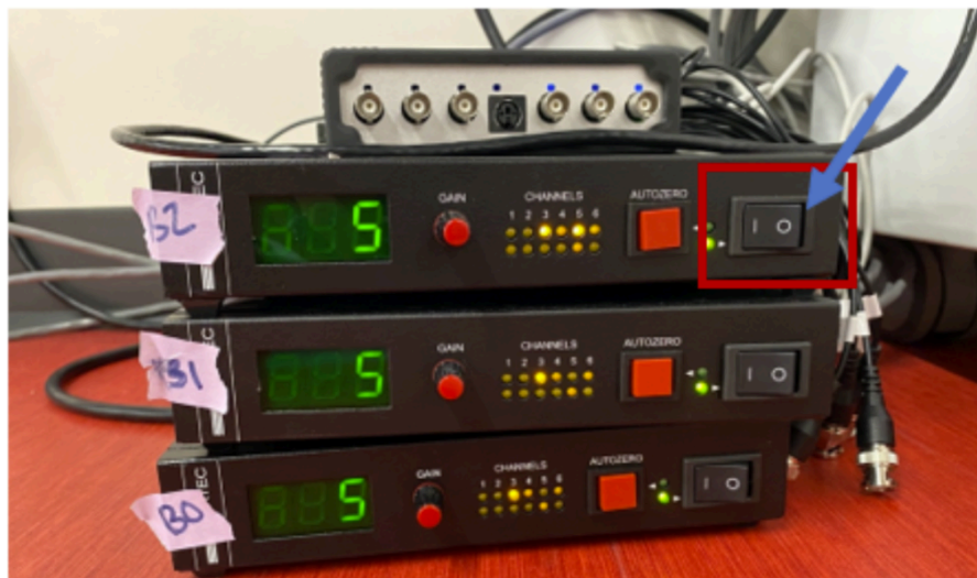
Figure 7: Amplifier boxes for in-ground force plates with indication of the power switch [o]
