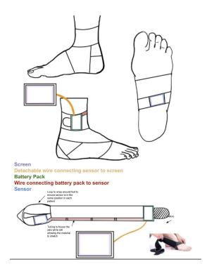
This device uses an ankle-brace like strip of elastic that can be adjusted to fit any patient. The loop at the end ensures that the sensor will sit in the same spot on each person's foot. The wiring will be fed through a tube of fabric to allow it to stay contained while the strap stretches. The battery pack will be fixed to the end of the strap, near the velcro strip. The wire connecting the battery pack/sensor to the readout will be detachable to prevent tangling when putting the device on.
