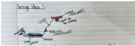
In this design, the weight bearing sensor would be resting in a cloth pocket. This would be placed under the client's foot. It would be attached with a wire to the Arduino circuit, which could rest in the shoe/boot. This wire would also attach to the screen that would display the weight data. This screen would be able to clip onto a patient walker if needed with a velcro strap.
