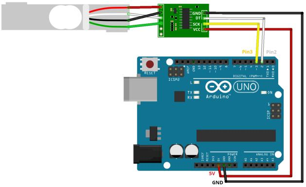
This circuit is the basic design for a load cell using an Arduino. The Arduino microcontroller is powered by a battery and is connected to a HX711 amplifier, which is a breakout board that allows you to easily read load cells to measure weight. This amplifier would be connected to a load cell, which measures the weight, and the measured weight would then be sent to the display.
