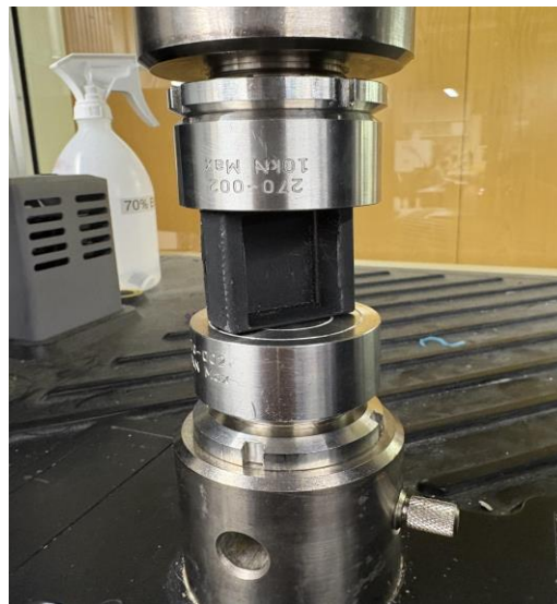
Figure [14]: MTS Testing Orientation of Device Watch Face with Resin Material
