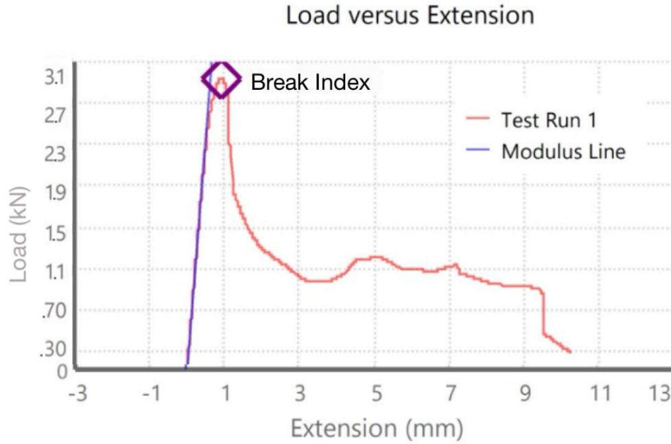
Figure [16]: Curve Showing Load (kN) vs Extension (mm) of PETG Material
