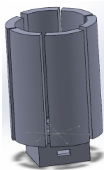
Figure 7. Expanding Pulley Mechanism CAD model side view.
