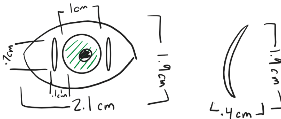
Figure 2: Drawing of 3D Printed Polymethyl Methacrylate Iris Conformer
