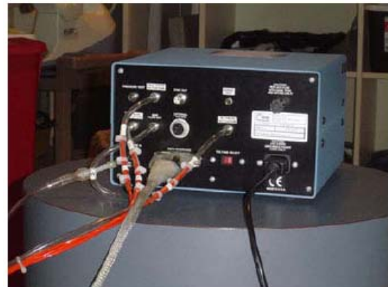
Figure 4. Current ventilator with gas lines (red) to run pneumatic valves.
