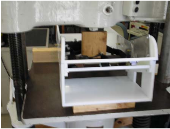
Figure 7: The setup for the hinge lock test is shown. A load was applied to the hinge to attempt to bend the locked seat.
