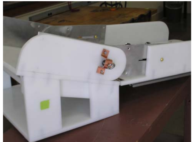
Figure 3: The pin locking mechanism is shown in this side view of the prototype. The back track can be seen under the back rest.
