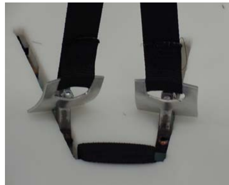
Figure 6: The testing setup for the strap anchor test is shown. A direct tensile load was applied to the straps.
