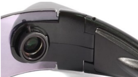
Figure 3: The Eyetop glasses project an image in the user's peripheral vision (above). Close-up of the imbedded screen (below).
