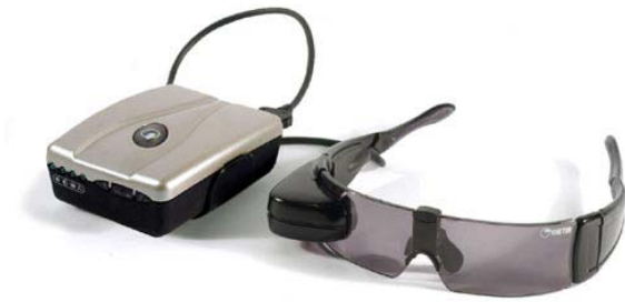
Figure 4: A wire connecting the control box to the glasses transmits images to the user.
