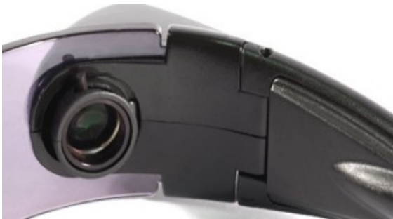
Figure 4: The Eyetop glasses project an image in the user's peripheral vision (above). Close-up of the imbedded screen (below).
