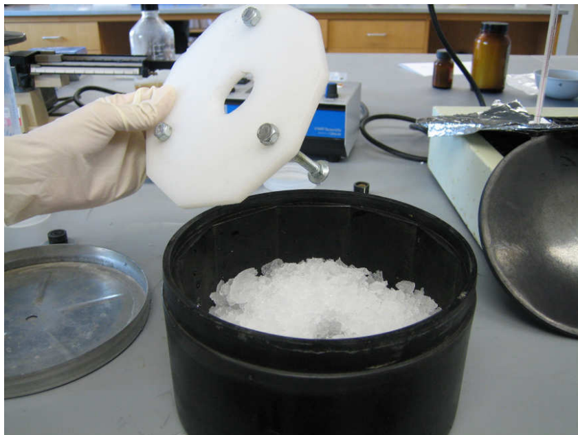
Figure 6: Prototype testing in Dr. Furgeson's lab. Shown is drum when filled ice for temperature testing.
