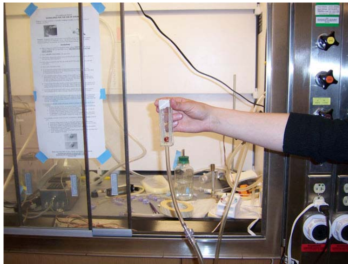
Figure 8: This picture shows the rotameter float failing to rise in spite of air flow through the tube
