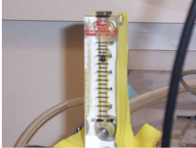
Figure 7: Calibrated rotameter used to find actual flow rate
