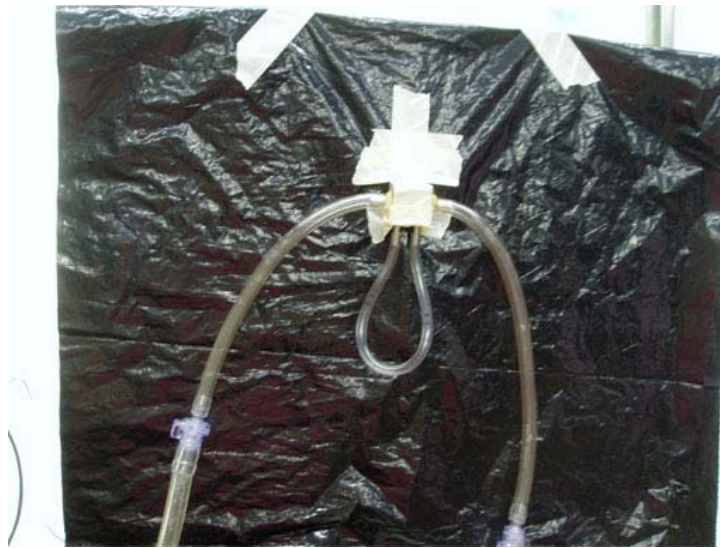
Figure 12: This picture shows our glued venturi meter tested in series with an accurate rotameter.
