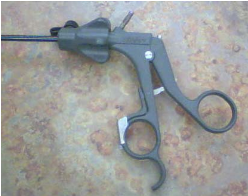
Figure 19. A mechanical advantage is produced by the lever.
