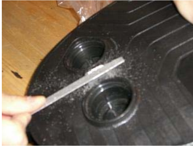
Figure 8: Sanding and Filing Bellows Pump
