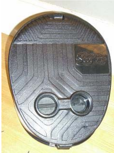
Figure 5: Top View of Sevylor Bellows Pump
