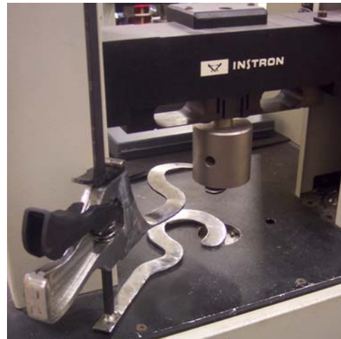
Figure 10. Load Testing : Using an Instron load cell, our device was tested in a worse-case-scenario.
