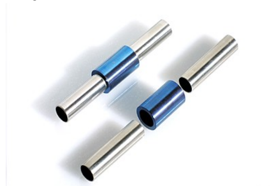
Figure 7- Cylinders of Nitinol are shown above. The proposed design would have the cylinders deformed to fit underneath the patient's ring and expanded to allow the ring to be removed.
