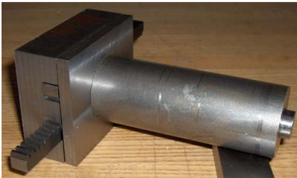
Figure 15d- Gearbox covered my face plate and grip around gear shaft
