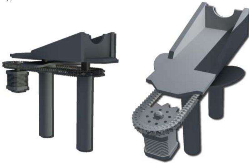
Figure 6. A computer generated image of Design 3, which rotates the experimental box, through a chain or belt, by a stepper motor which is placed outside of the electromagnetic field.
