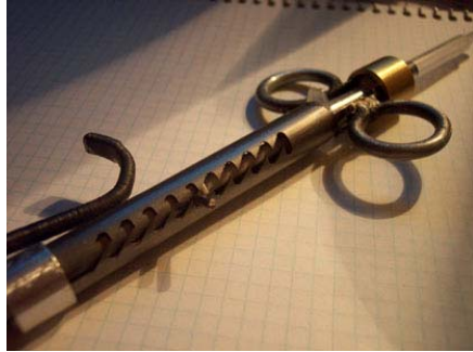
Fig. VI: The Step-Meister 1.0 Our design from last semester incorporated an increment size that was controlled by a diagonal groove.
