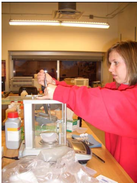
Figure XIV : Increment Volume Testing Water is expelled and each increment size is recorded by an analytical balance
