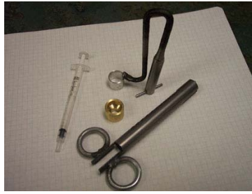
Fig. VI: The Step-Meister 1.0 Our design from last semester incorporated an increment size that was controlled by a diagonal groove.
