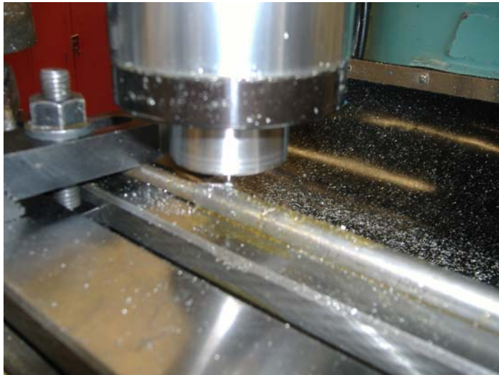
Figure X : CNC Milling Machine CNC machine milling the groove onto the tube of our device
