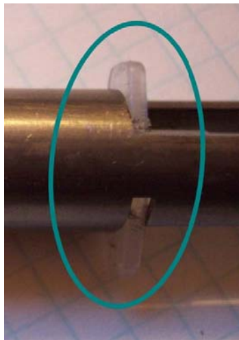
Fig. XII: Friction Fit Slot . The syringe's finger grips, circled, rotate into a friction fit slot that keeps the syringe from falling out.
