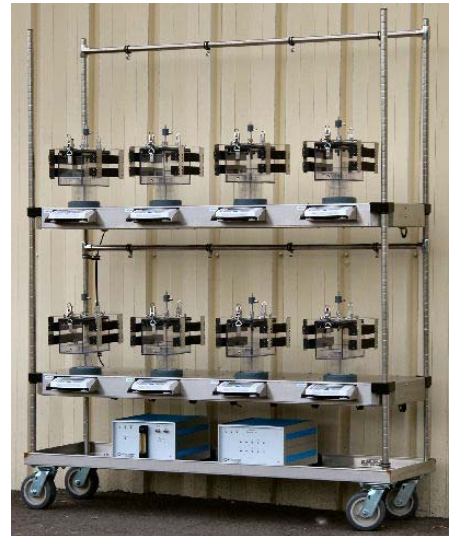
Figure 2: The CLAMS system. This is a state of the art indirect calorimetry system [4].
