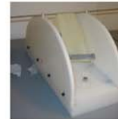
Figure 3. First prototype processing dermis. The rod is moved back and forth along the tracks by an operator.
