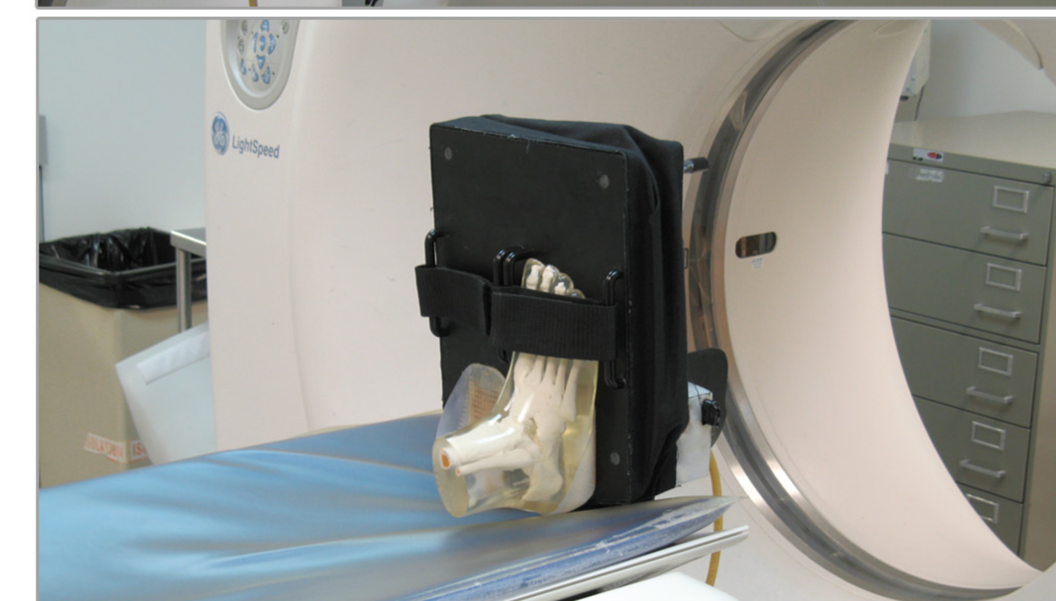
The device attached to a CT table with a phantom foot strapped in. When run through a scan, the device generated no noticeable image artifacts.
