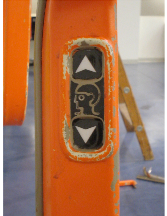
Figure 2: The controls on the Hill-Rom bed are small, completely flat and hard to keep activated. They are located on the inside of the hand rail on both sides of the bed. Immediately below the bed back angle control (left), is the foot control. Having the two in close proximity makes it easy to activate the wrong control system.
