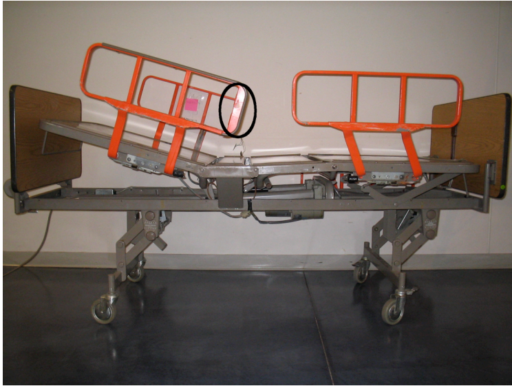
Figure 1: Hill-Rom hospital bed acquired for project. The head of the bed is slightly raised in this picture, and the location of the bed-back angle and foot position controllers on the hand rail have been circled in black.
