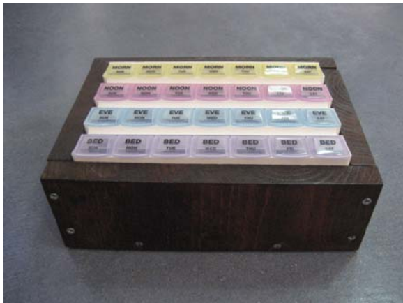
Figure 1. Electronic Medication Adherence Device (EMAD): a pillbox with a circuit to monitor the opening of the compartments. The circuit is held within the wooden box to ensure the patient is not apprehensive about using the box.
