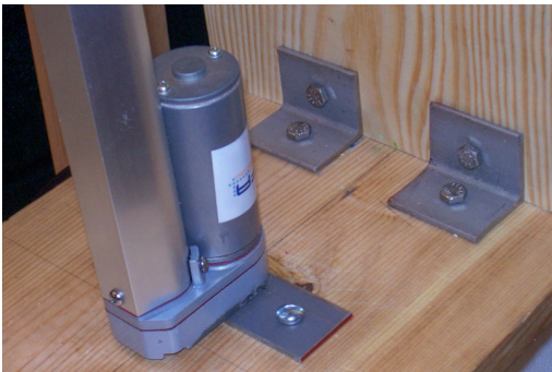
Figure 8: Base of linear actuator with metal flange.
