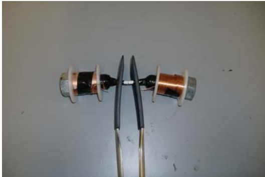
Figure 21: When the needle is on one side of the device with that electromagnet holding it in place. The clamp is then closed until the two sides meet. The power supply is then applied to the opposing electromagnet and the clamp is released leaving the needle in the opposite side.
