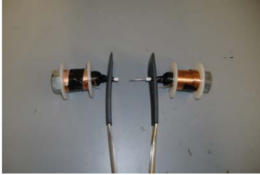
Figure 21: When the needle is on one side of the device with that electromagnet holding it in place. The clamp is then closed until the two sides meet. The power supply is then applied to the opposing electromagnet and the clamp is released leaving the needle in the opposite side.
