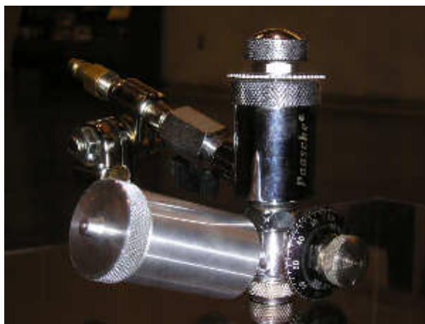
Figure 10: Paasche© A-AU automatic spray gun and corresponding flat spray nozzle operate at a minimum of 50 psi, supplied through the pipe nipple pictured in the background. Flow rate is determined by the black hand valve, also located on the pipe nipple. The attached matrix reservoir can hold up to three ounces of liquid to allow for multiple coats without refilling.
