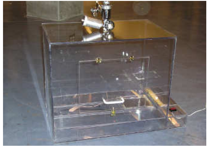
Figure 6: Front view of the enclosure, supporting the sprayer through a \frac{5}{8} " hole in the top panel and the plate conveyor on a panel mounted 2" from the floor. The smaller rectangular box at right is the motor cavity, and the larger enclosed area houses the conveyor and spraying process.
