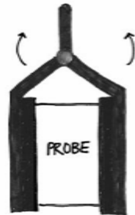
Figure 6. Proposed shape of the foam plate probe holder, with arms that swing up to release the probe.
