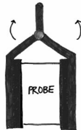
Figure 7. Proposed shape of the foam plate probe holder, with arms that swing up to release the probe.
