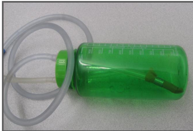
Figure 6. The assembly of the collection vessel with the inclusion of the one-way valve.
