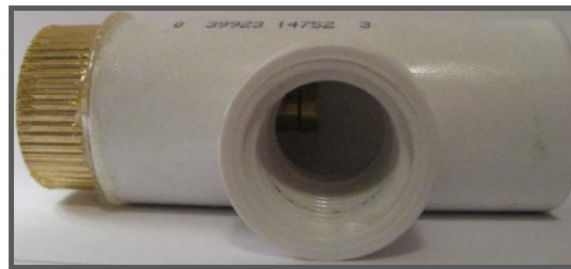
Figure 8. The nozzle is inserted so that the jet portion is located at the interior of the tee.
