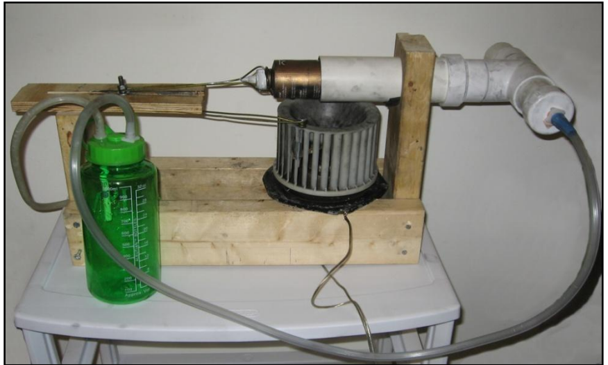
Figure 4. The image above displays the final design, including the fan motor, piston arrangement, and collection flask.
