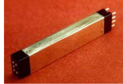
Figure 10: Microsolenoid driven Braille cell, used by researchers at MIT. http://web.mit.edu/erblan/www/Graphics/solenoid-big.jpg
