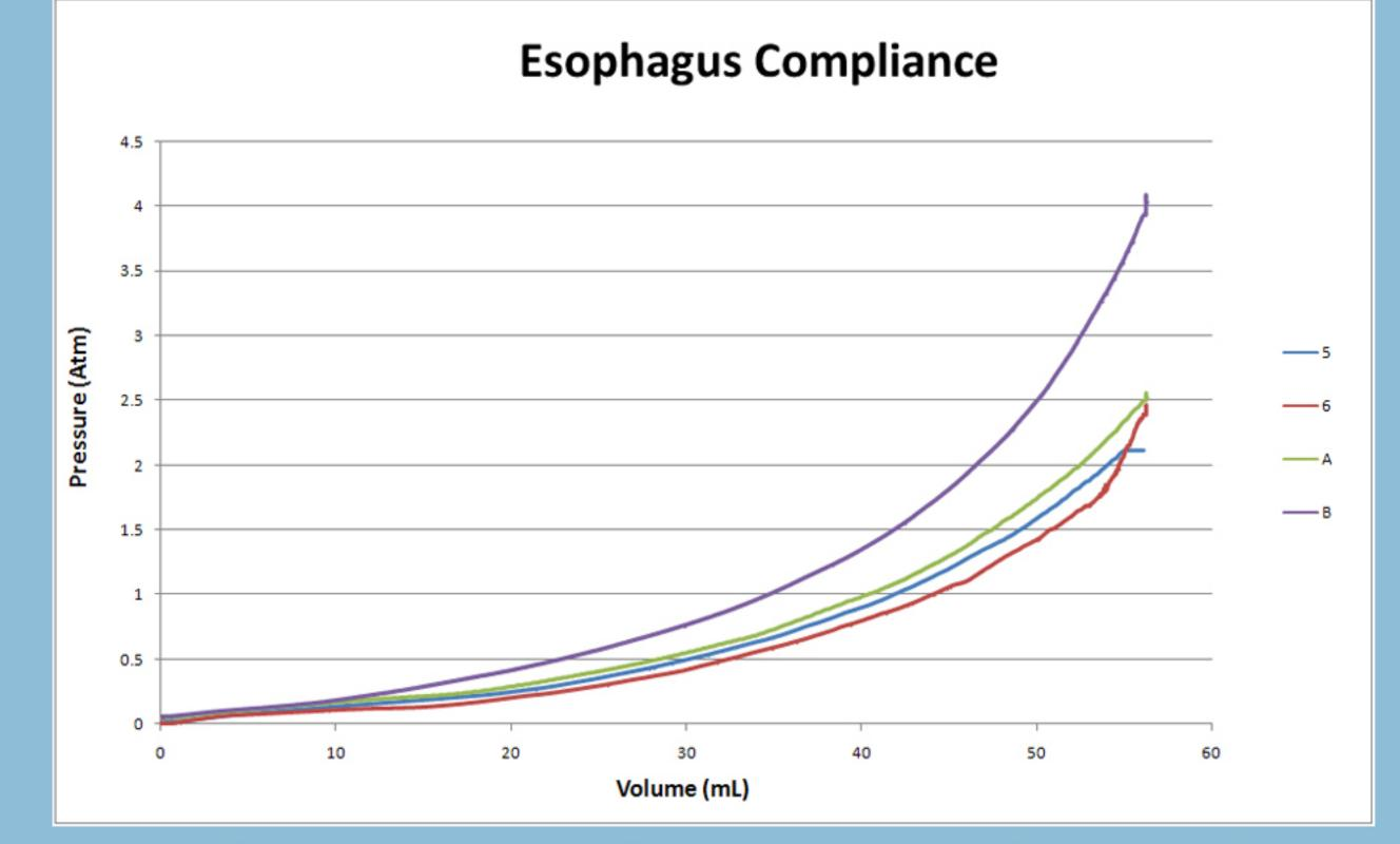
Figure 8: Compliance data from esophagi 5,6, A and B. Esophagus 5 had a thickness of 1.21 mm and diameter 15.02mm, esophagus 6 had a thickness of 0.94 mm and diameter 20.28mm, esophagus A had a thickness of 1.58 mm and diameter 16.05 mm, and esophagus B had a thickness of 1.02 mm and diameter 8.21 mm.
