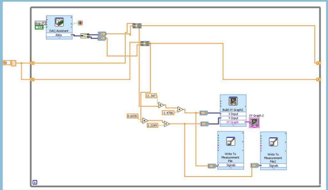
Figure 4: The LabVIEW program used to acquire the voltage data, convert to units of pressure and volume and display a real time compliance graph.
