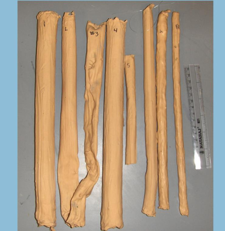
Figure 6: The eight liquid latex esophagi constructed for testing the device.
