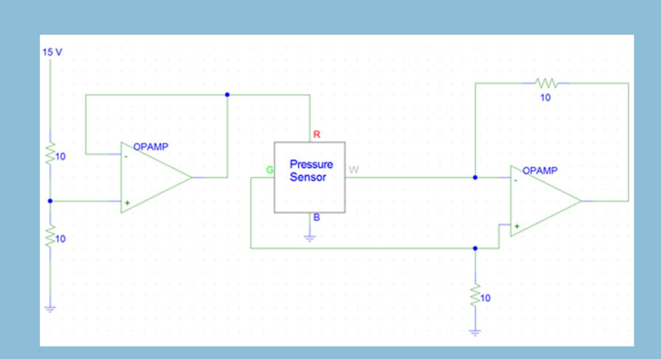
Figure 5: The circuit used to amplify the pressure sensor output voltage.
