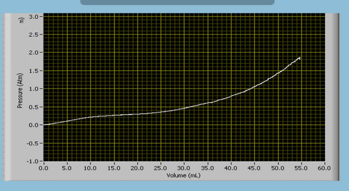
Figure 7: The compliance graph made with LabVIEW. The x-axis is calibrated in milliliters and the y-axis is calibrated in atm. Pressure was applied to the balloon causing it to inflate.
