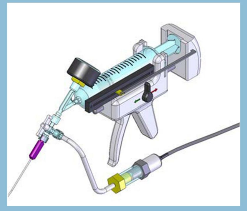
Figure 3: The current setup consists of a syringe gun with a linear potentiometer attached to its side to measure the change in volume. A pressure transducer attaches at a T -joint to measure the pressure in the balloon
