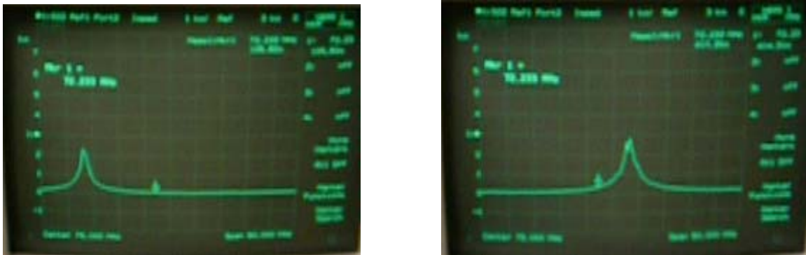
Figure 3. Resonant frequency peaks measured on oscilloscope.
