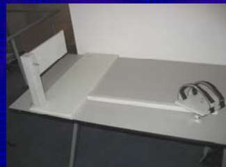
Figure 6: Our design showing pannus retractor and leg rod attached to the bottom board.
