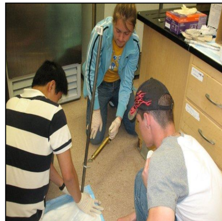
Figure 19: Application of Horizontal Force to Cranial Pedestal 3 Inches above Monkey's Skull
