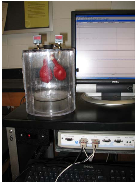
Figure 5. Respiratory model connected to BioPac® system.
