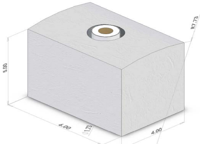
Figure 12: A representative portion of the rubber mold model. The entire model is made of a single soft polyurethane. All measurements are in inches.
