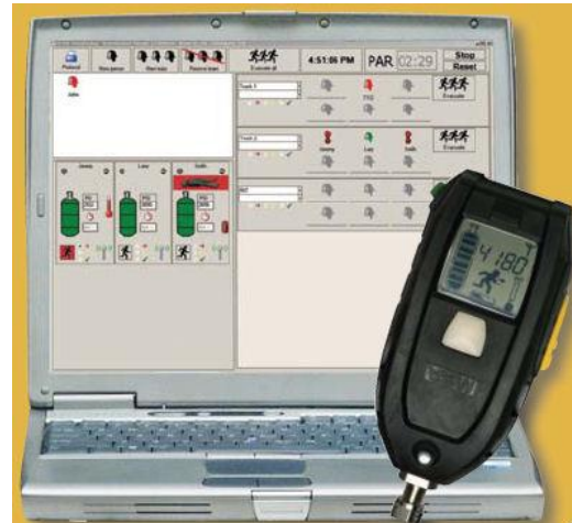
Figure 2 - The MSA TxR ICM® Accountability System. The unit with the computer is the sensor and also serves as a miniature display. (MSA, Inc., 2006 )
