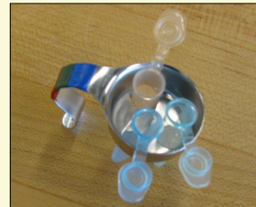
Figure 5. Eppendorf holder fabricated for holding three Eppendorfs.
