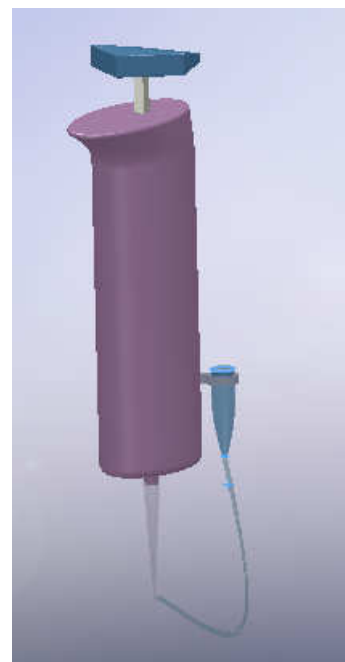
Figure 6: Flexible straw design with reservoir attached to body of shortened pipette and straw reaching to end of pipette tip.
