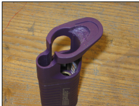
Figure 13. Standard micropipette grip with internal components removed and notch cut out for MiniFix.
