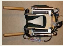
Picture 4 shows the face cradle as viewed from below. The tracks and pistons allow pneumatic actuation.
