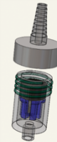
Figure 2: Final prototype. The cage (blue), stopper (black) and ball (grey) are all inside a cylinder with threaded (green) cap. See Figure 6 for dimensions and Figure 5 for final prototype. At the bottom of the cylinder is a connection for the specimen trap and at the top, the cap connects to the vacuum tubing.
